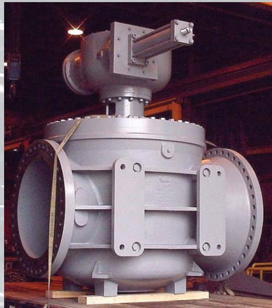
This Ø24" cone valve (above) is controlled by a Ø6" x 14" stroke actuator with a 2" stroke adjustment, stainless steel rod and special protective paint.
