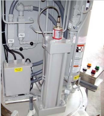
This  $\varnothing 5''$  x 32.00'' stroke actuator has a  $\varnothing 2''$  rod and is equipped with full stroke position indication to determine percentage of valve positioning.
