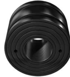
Standard glass-filled Teflon, O-ring energized piston seal with two bronze-filled bearing strips—installed on a ductile iron piston. (Code G)
